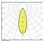
**Scheda tecnica Ledvance Downlight LED Performance Nero 8W 650lm 40D - 830 Luce Calda | 90x83mm**
