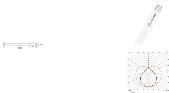
**Scheda tecnica Ledvance Tubo LED T8 EM Ultra Output Value Conventional (EM), Mains (AC) Ultra Output 20W 2400lm - 865 Luce Del Giorno | 120cm - Sostitutiva 36W**
